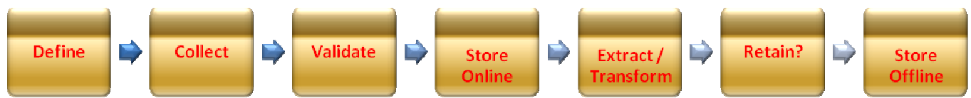
Figure 4 – Flow structure of data in the warehouse managed by ETL codes.
